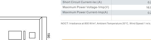
**MECHANICAL DATA** Solar cells Poly-crystalline 39\*26mm Cell configuration 36 cells(4X9) 190\*300\*17mm Module dimensions 0.68KGS Weight Front Cover 3.2mm Tempered Glass Frame Material Anodized Aluminum Alloy J-BOX IP65 or IP67, 1 Diodes Cable 0.5mm<sup>2</sup>(IEC), 800mm
